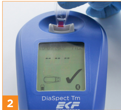
2 Insert the filled cuvette and press down gently. Remove the cuvette immediately after the first beep tone
