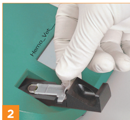
Put microcuvette into analyser.
