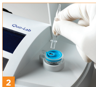
2 When prompted press reagent bead into cartridge using the reverse end of the sampling tool.
