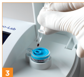
3 Insert sample tool into cartridge and snap off handle.
