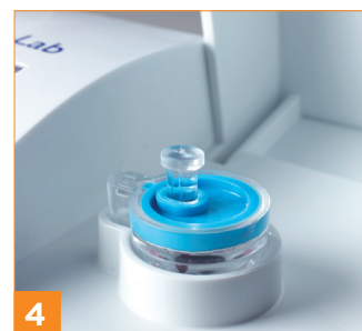
4 Close analyser lid. Result displayed within 4 minutes.
