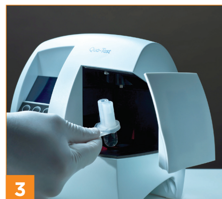
Insert cartridge into analyser. Results displayed within 4 minutes.
