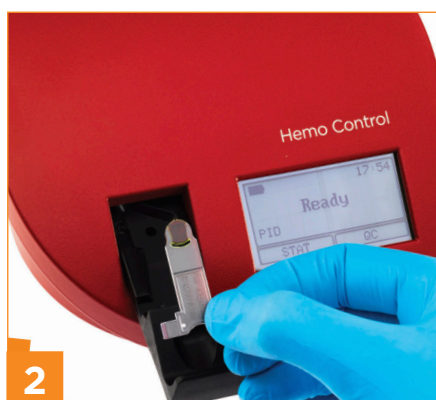
2 Put microcuvette into analyzer.
